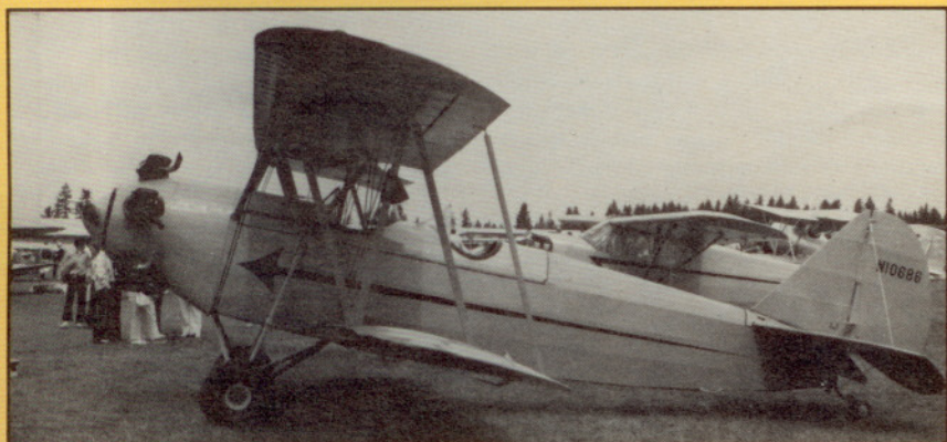
Originally, the Student Princes were equipped with Cirrus engines, but this picture shows N10686 with a more powerful Kinner engine and a war-surplus Ryan PT-22 propeller spinner.
