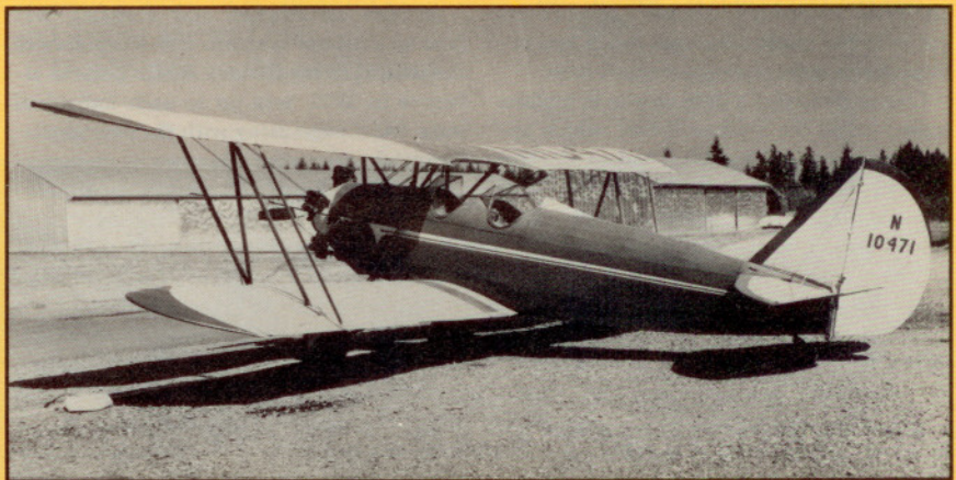
Before and after: The 1954 photo above shows early modifications that include a Kinner engine; it was not till 1963 that this Student Prince received the 220-hp Continental. At the same time the rudder was enlarged, as was the center cutout for easier access to the cockpit.
