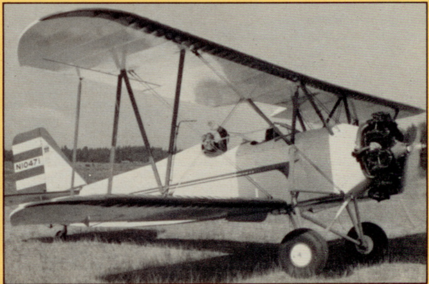
Before and after: The 1954 photo above shows early modifications that include a Kinner engine; it was not till 1963 that this Student Prince received the 220-hp Continental. At the same time the rudder was enlarged, as was the center cutout for easier access to the cockpit.
